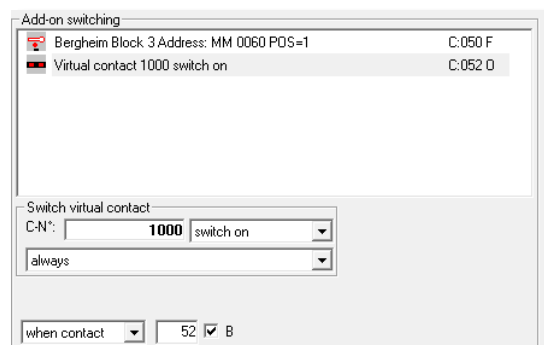
Fig. 7.91 The "Switch virtual contact" follow-up switching.
