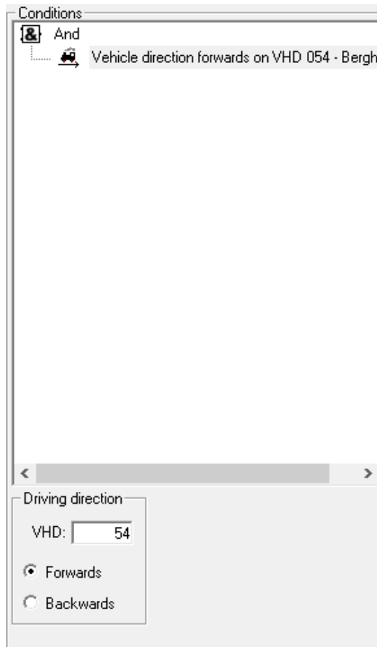
Fig. 13.10 The condition “Vehicle direction on VHD”
