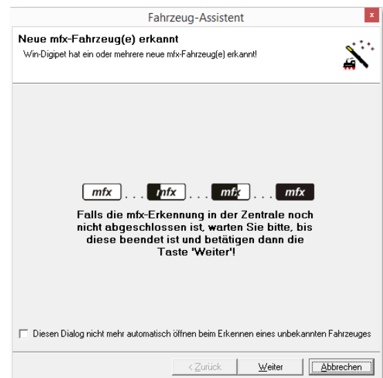
Fig. 4.74 30 vehicle assistant has recognised a new mfx vehicle. (Picture in German language)
