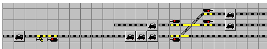
Fig. 3.74 Placement of different types of a vehicle display in the track diagram editor
