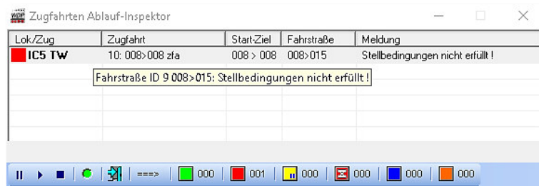
Fig. 7.6 Tooltip showing the reasons for the current red stat in the tour event inspector
